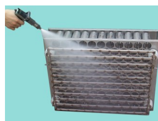
Figure 4-2 Pulverize as células de favo de mel.
